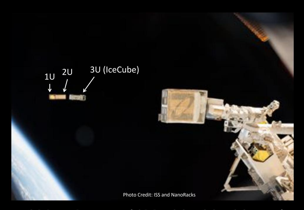
3U cubesat (1U=10x10x10 cm), 883 GHz cloud radiometer (launched 2017)
